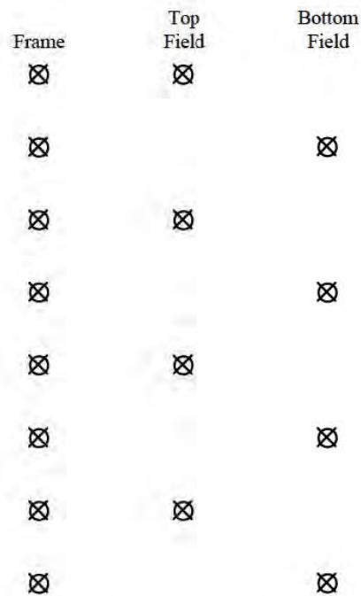
Figure 6-6 — Vertical positions of samples with 4:2:2 and 4:4:4 data
