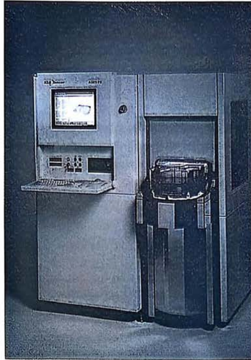
Fig. 8-31 Photograph of an automated thin film thickness measuring system. Courtesy of KLA-Tencor.
