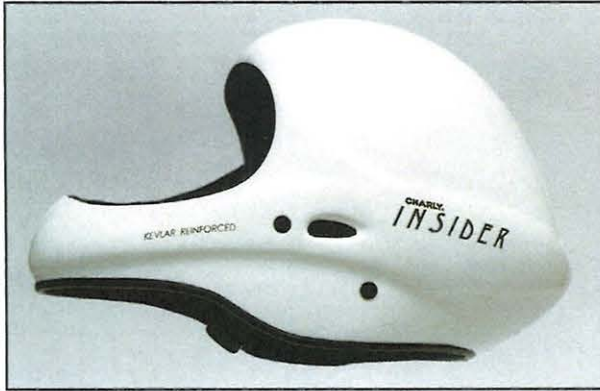
A popular helmet amongst hang glider pilots is this stylish unit, the Charly Insider. The outer shell is made from a Kevlar fiber glass composite and the interior is EPS foam. It does not come with any form of visor or faceshield. Photo courtesy of Gene Atkins, Wills Wing.
