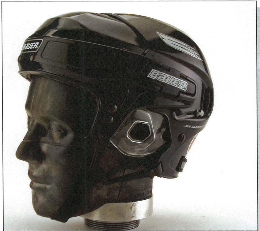
Bauer HH8000. Similar in many ways to the HH5000, it employs an ABS shell and the liner is triple density expanded polypropylene bead foam. Both models are certified to CSA and CE. Photographed by Stephen Fenn.
