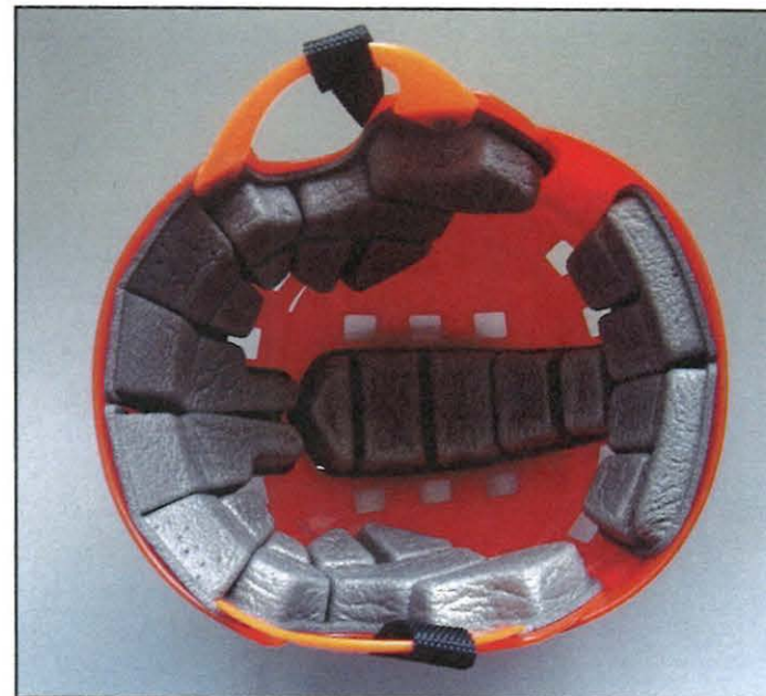
Jofa padded interior. Not bad, but not good enough to meet the new CSA standard of the time.
