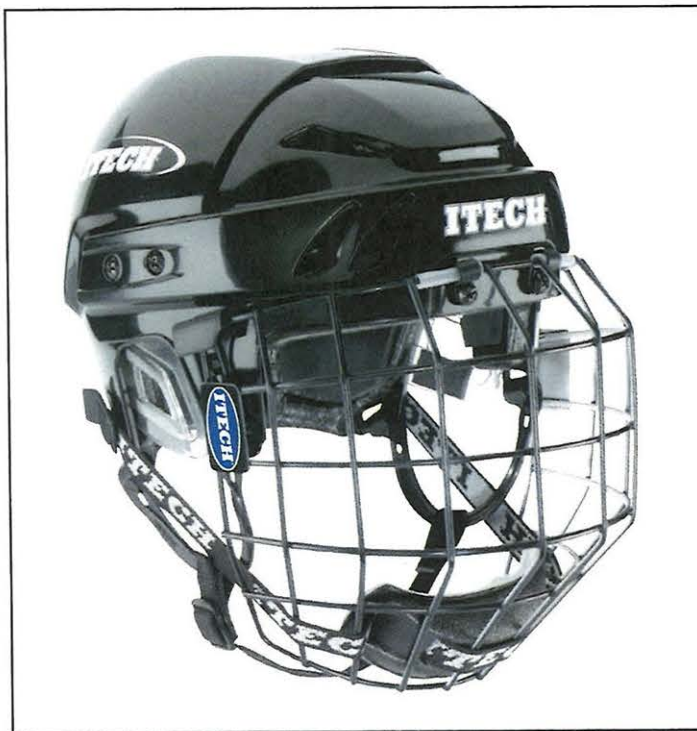
Itech HC100 with wire face guard. The HC100 also employs a two-piece shell. For impact energy absorption it uses expanded polypropylene EPP bead foam. The comfort liner is made of a Pro Gel Foam material. The ear pieces are removable.
