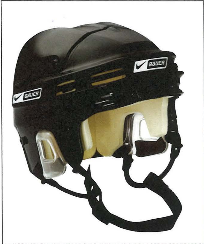
Nike Bauer 4500. Like many of its competitors, Nike Bauer brand hockey helmets' shells are injection molded high density polyethylene HDPE. This Nike Bauer model 4500 employs two layers of vinyl nitrile foam for energy absorption.
