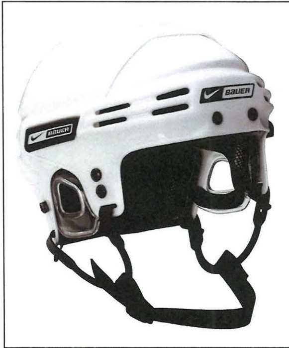
Nike Bauer 5500. The 5500 model actually uses EPP foam in three different densities. The shell is available in three different sizes to accommodate a wide range of head shapes.
