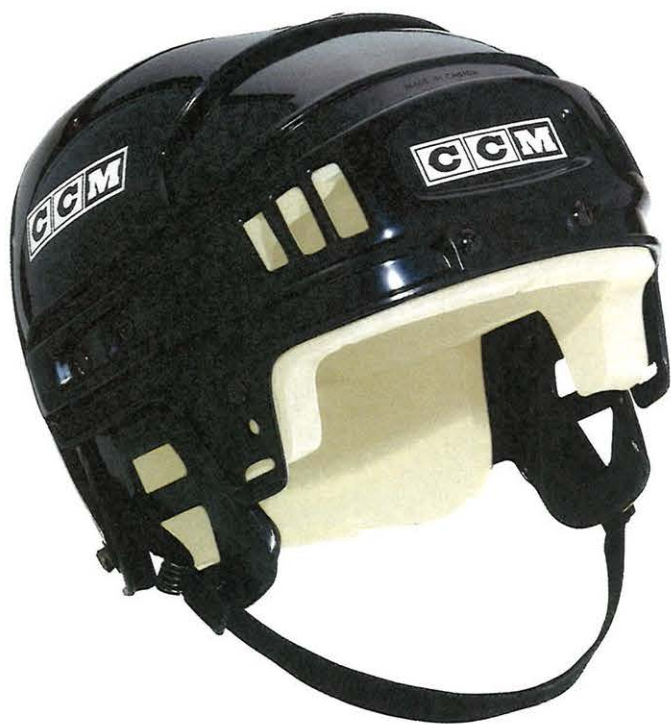
CCM 492. A single density die-cut vinyl nitrile liner in a molded HDPE two-piece shell. The Proguard look lives on.
