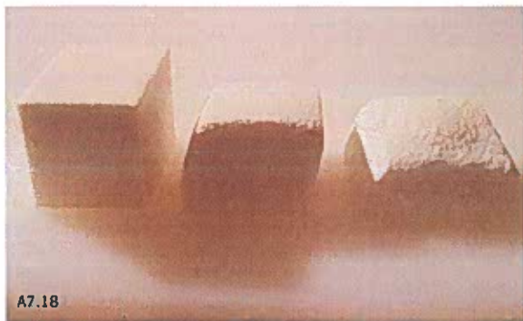
Fig. A7.18 The cubes of modeling clay are flattened by 90 minutes of vacuum therapy. From left to right: 0 mmHg, 75 mmHg, 200 mmHg of applied suction.
