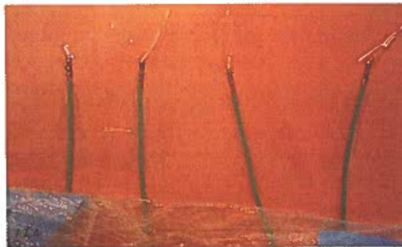
Fig. A7.4 Placement of the four measurement probes on a flat desktop. Fixation of the unidirectionally constructed probe tip using tape strips to prevent unplanned rotation of the probe.
