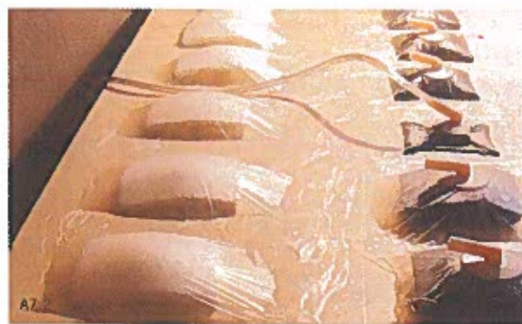
Fig A7.2 Experimental design for demonstration of the effect of suction applied to a cube of modeling clay in relation to the suction strength. Each cube was exposed to suction applied through one of the two types of foams over a period of 90 minutes.
