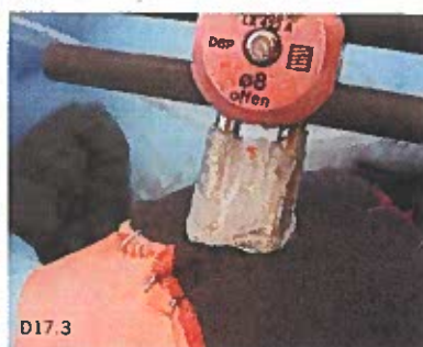
Fig. D17.3 Apply a strip of gel to the screws. Completely cover and connect both screws with a layer of gel.
