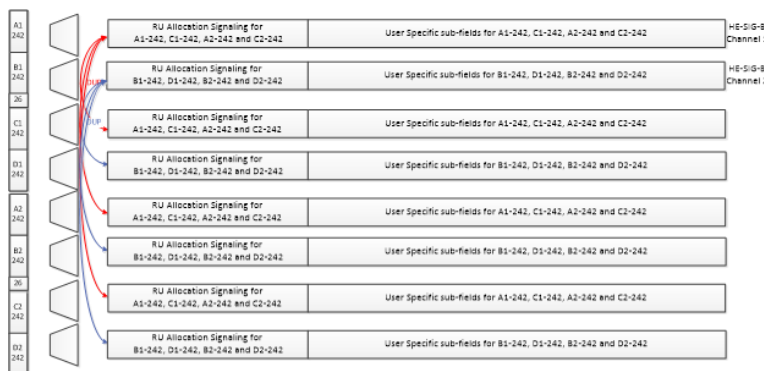
Figure 26-27 - Default mapping of the two HE-SIG-B channels and their duplication in a 160 MHz PPDU
