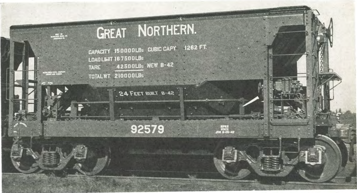
Fig. 2.666—Great Northern 75-ton capacity hopper iron ore car. Series 90,000-92,999. Builder, Bethlehem Steel Company.
