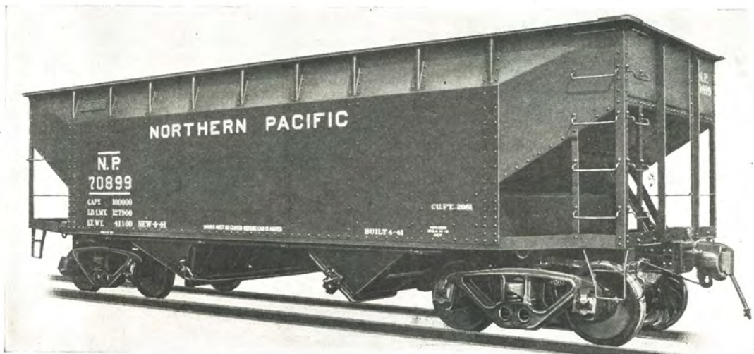
Fig. 2.614—Northern Pacific 50-ton twin hopper coal car. Builder, American Car and Foundry Co.
