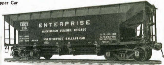
Fig. 2.680—55-ton Multi-Service Car
