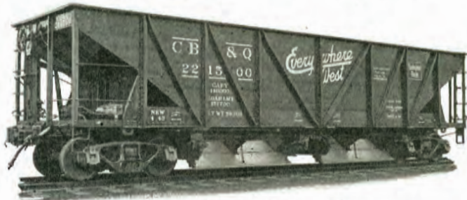
Fig. 2.681—70-ton Multi-Service Car
