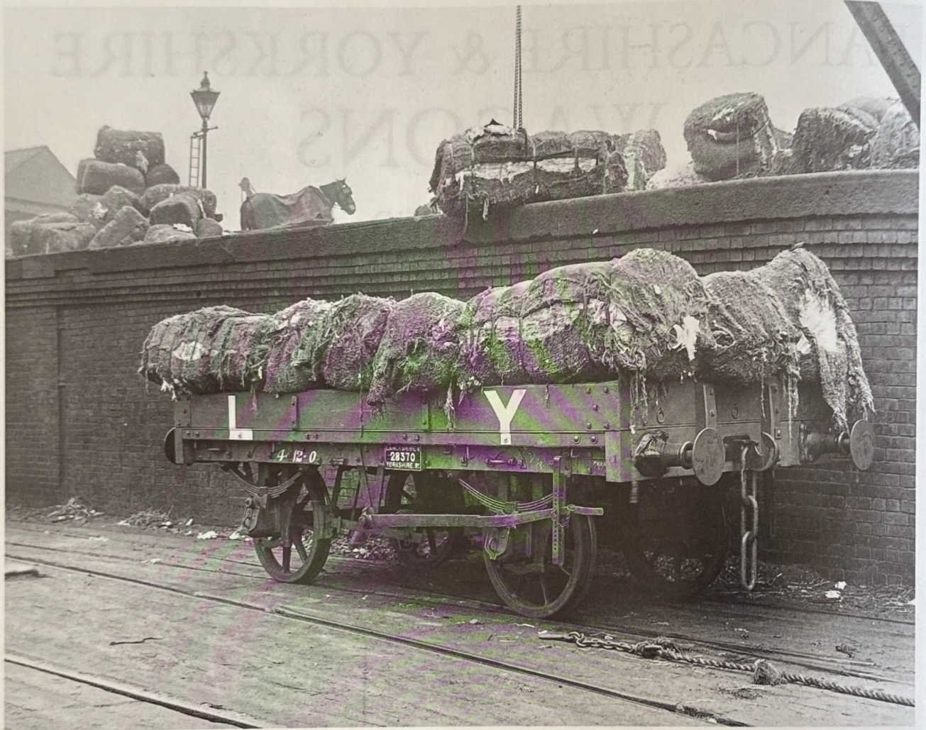
Plate 157. The vast majority of merchandise went by open wagon (often sheeted over to keep out the elements) and this view of a Dia. 1 single planker is typical, except that the wagon looks so clean. The paint date on the solebar says 2/16 and the photograph is dated 16th March 1916 which explains why; this older style narrow side rail vehicle had received new headstocks (and oil axleboxes probably) during the recent general repair, some 20 years after building. The wagon also features in the bottom right-hand corner of Vol. 1, Plate 112.
