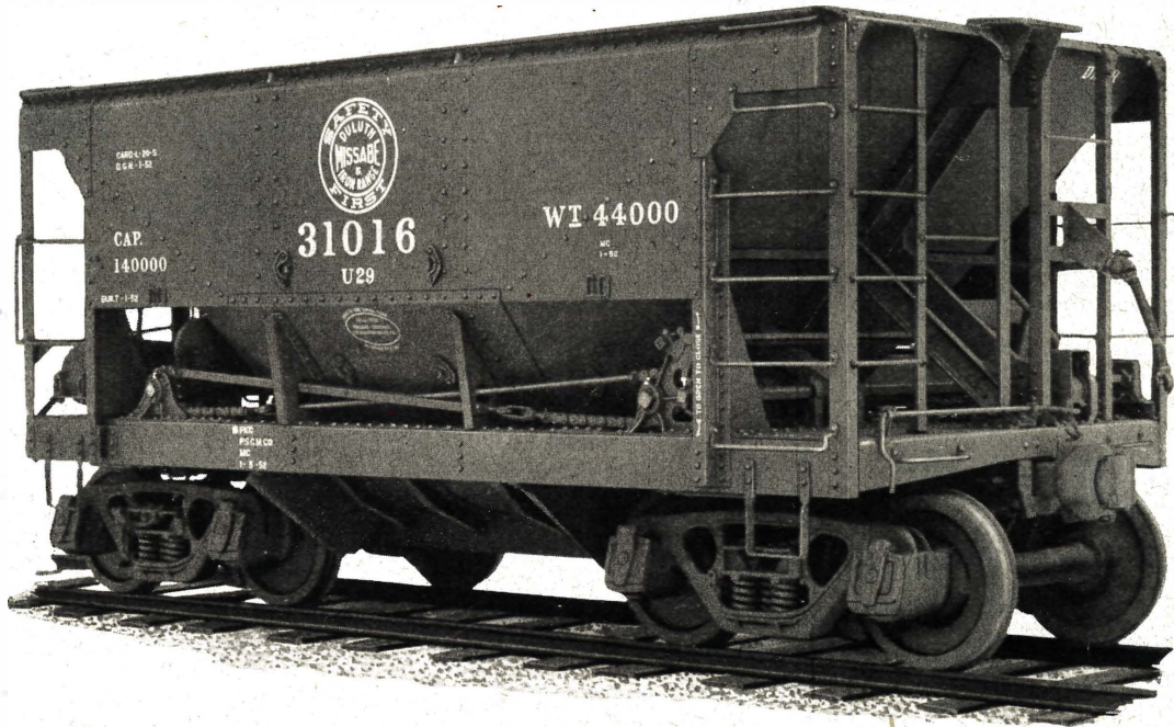
70-ton Center Discharge Ore Car.
