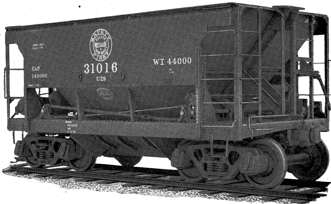
70-ton Center Discharge Ore Car.
