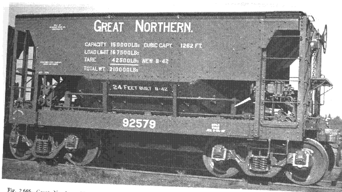
Fig. 2.665—Great Northern 75-ton capacity hopper iron ore car. Series 90,000-92,999. Builder, Bethlehem Steel Company.
