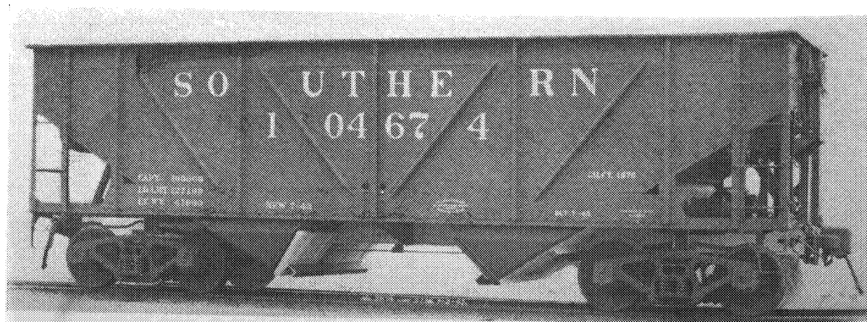
Fig. 2.618 —Southern Ry. 50-ton composite twin hopper coal car. Builder, Pullman-Standard Car Manufacturing Co. Light weight, 41,900 lb.; load limit, 127,100 lb.; capacity, 1,970 cu. ft.; length inside, 33 ft. 0 in.; width, 9 ft. 6 in.; height of sides, 10 ft. 8 in. (A. A. R. Emergency 1942 Design—For drawing see 1943 Car Builders' Cyclopedia , Page 249) Description: Railway Age , Aug. 28, 1943
