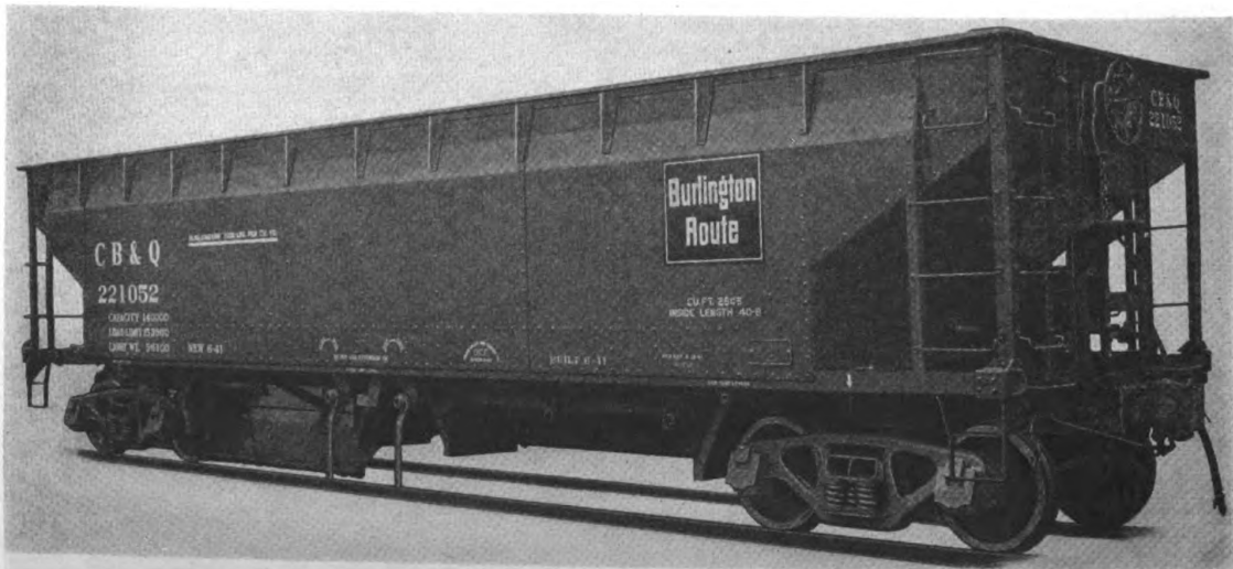
Fig. 2.659 —Chicago, Burlington & Quincy 70-ton Hart selective ballast and coal car. Light weight, 56,100 lb.; load limit, 153,900 lb.; capacity, 2,505 cu. ft.
