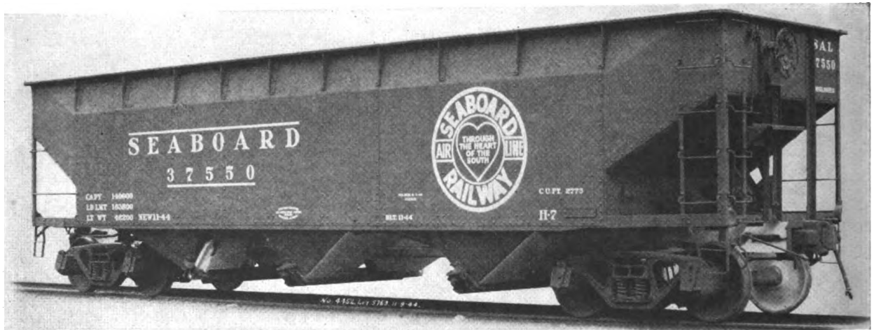
Fig. 2.628 —Seaboard Air Line 70-ton triple hopper car. Road Class H-7. Builder, Pullman-Standard Car Manufacturing Co. Light weight, 46,200 lb.; load limit, 163,800 lb.; capacity, 2,773 cu. ft.; inside length, 40 ft. 8 in.; width, 10 ft. 4 in.; height of sides, 10 ft. 8 in.
