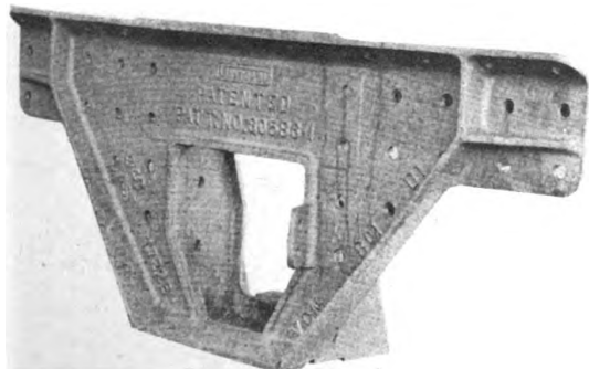
Unitcast Body Bolster Center Casting
