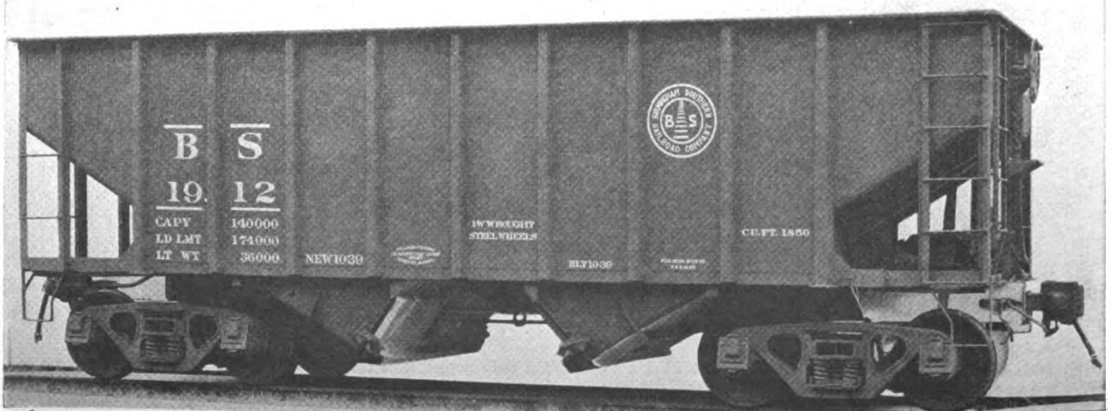
Fig. 2.624 —Birmingham Southern 70-ton light-weight twin-hopper car for coal or ore service, A. A. R. Class HM. Builder, Pullman-Standard Car Manufacturing Company.
