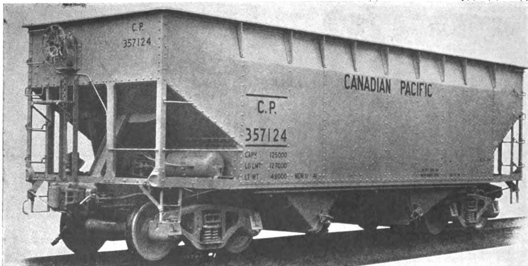
Fig. 2.622 —Canadian Pacific 125,000 lb. capacity twin hopper car. Built for National Steel Car Corporation. Capacity, 2,190 cu. ft.; light weight, 42,000 lb.; load limit, 127,000 lb.; length inside, 33 ft. 0 in.; width inside, 10 ft. 4 in.; height overall, 10 ft. 10 in.
