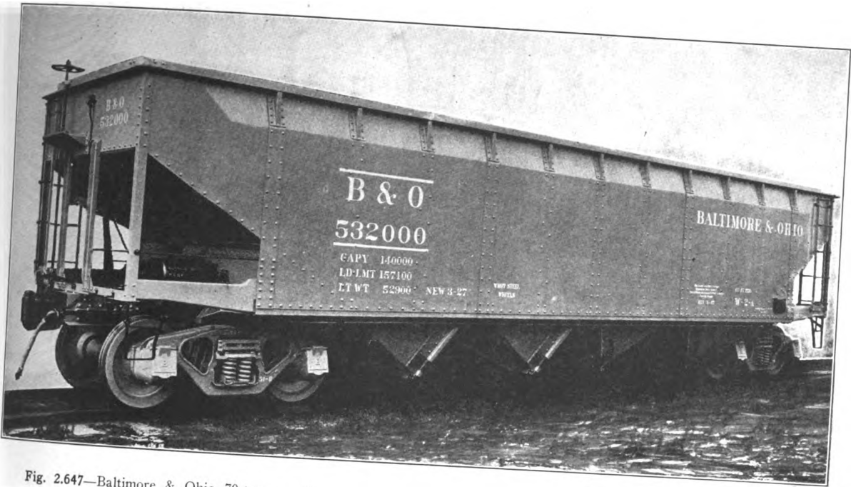
Fig. 2.647—Baltimore & Ohio 70-ton capacity quadruple hopper coal car, Road Class W-2-A, A. A. R. Class HT. (See also Figs. 2.646-2.648)
