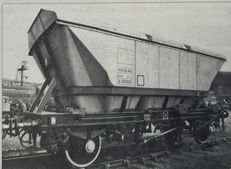
An official view of B350001. This is the second prototype, built to diagram 1/157 and coded HOP 32 AB. Tare weight: 11ton 4cwt. (Author's Ref No W50069/BR)
