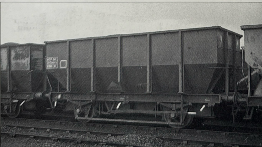
B338121 at Mansfield, Notts in 1970. This lot 3525 wagon is in original condition, including the yellow triangle. Although unfitted, freight brown livery was applied as per the specification when the wagons were ordered from Pressed Steel Ltd. Tare weight: 10ton 15cwt. (Courtesy Eric Gent)
