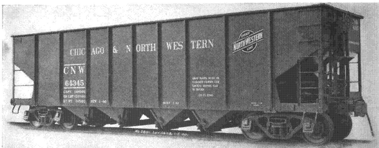
Fig. 2.651 —Chicago & North Western 70-ton capacity quadruple hopper car, A. A. R. Class HT. Builder, Pullman-Standard Car Manufacturing Company.
