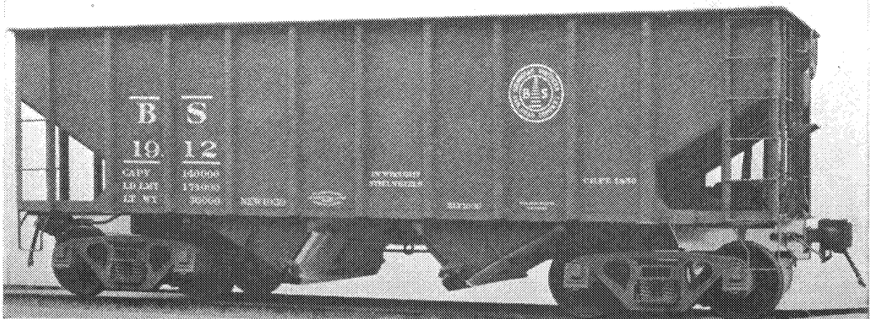
Fig. 2.624 —Birmingham Southern 70-ton light-weight twin-hopper car for coal or ore service, A. A. R. Class HM. Builder, Pullman-Standard Car Manufacturing Company. Capacity, 1,850 cu. ft.; light weight, 36,000 lb.; load limit, 174,000 lb. Inside, length 30 ft. 3 in.; width 9 ft. 7 in.; height of sides, 10 ft. 8 in.
