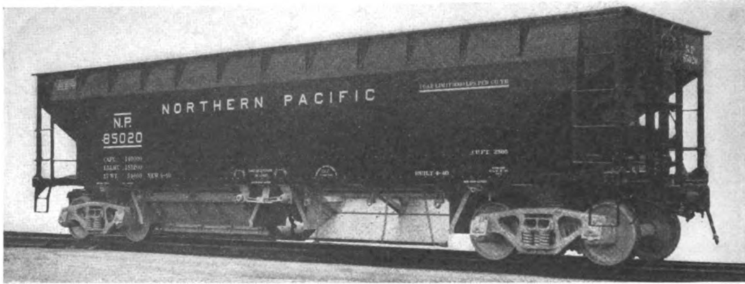
Fig. 2.657 —Northern Pacific 70-ton Hart selective ballast and coal car. Light weight, 54,800 lb.; load limit, 155,200 lb.; capacity, 2,505 cu. ft.; inside, length 40 ft. 8 in.; width 10 ft. 1 in.; height of sides 10 ft. 8 in.; length over strikers 41 ft. 8 in.
