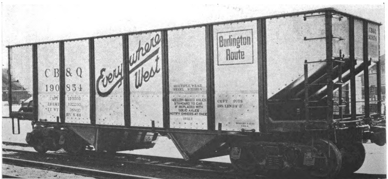
Fig. 2.615 —C. B. & Q. 55-ton aluminum twin hopper coal car. Rebuilt on old steel frame. Built at Havelock shops.
