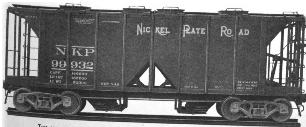
Two compartment covered hopper car for the Nickel Plate. Nominal capacity, 140,000 lb., or 1,958 cu. ft., with light-weight of 52,300 lb. Load limit, 157,700 lb.
