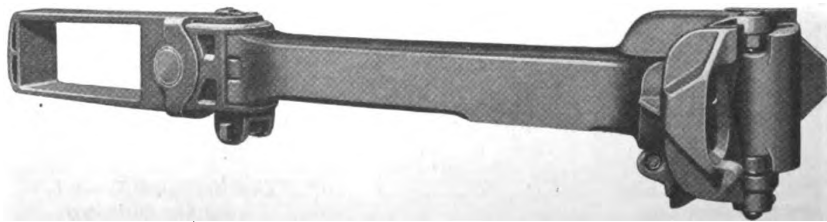
Fig. 10.111 —A.A.R. Tightlock Coupler, Yoke and radial connections for passenger car service.
