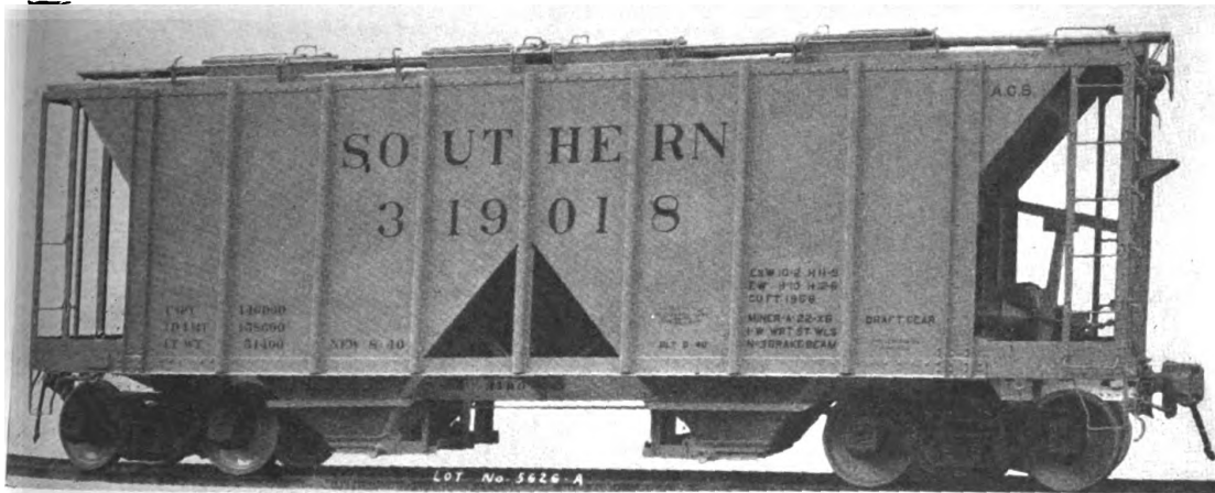
Fig. 2.693—Southern Railway 70-ton covered hopper car. Builder, Pullman-Standard Car Manufacturing Co. Capacity 1,958 cu. ft.; light weight 51,400 lb.; load limit 158,600 lb.; inside, length 29 ft. 3 in.; width 9 ft. 5 in.; height to top of running board 12 ft. 10 in.
