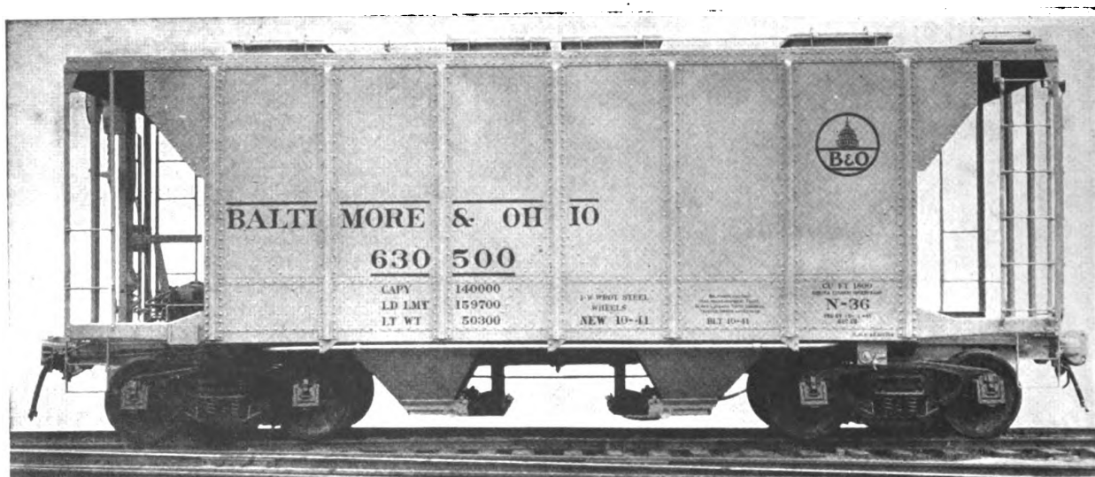
Fig. 2.683 —Baltimore & Ohio 70-ton bulk cement hopper car with Duryea cushion underframe. Road Class N-36, A. A. R. Class LO. Light weight, 50,300 lb.; load limit, 159,700 lb.; capacity, 1,800 cu. ft.; axle journals, 6 in. x 11 in. Built by Greenville Steel Car Co.
