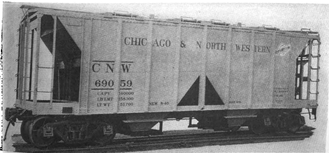
Fig. 2.694—Chicago & North Western 70-ton covered hopper car. Builder, General American Transportation Corp. Capacity 1,958 cu. ft.; light weight 51,700 lb.; load limit 158,300 lb.; inside, length 29 ft. 3 in.; width 9 ft. 5 in.; height over running board 12 ft. 10 in.
