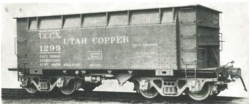
Fig. 2.671—Utah Copper Company 200,000-lb. capacity high-tensile steel, flat bottom, ore car. Unloaded by car dumper. Builder, Pressed Steel Car Company, Inc. Light weight, 48,500 lb.; load limit, 202,500 lb.; capacity, 1,640 cu. ft.; inside, length 24 ft. 5 in.; width 10 ft. 6 in.; height 6 ft. 6 \frac{5}{8} in. Description of earlier lot: Railway Age, October 30, 1937
