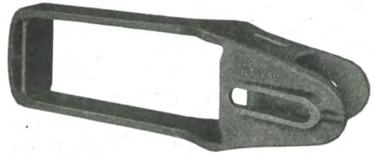
Fig. 10.100—Buckeye A.A.R. vertical-plane draft yoke of high-tensile steel.
