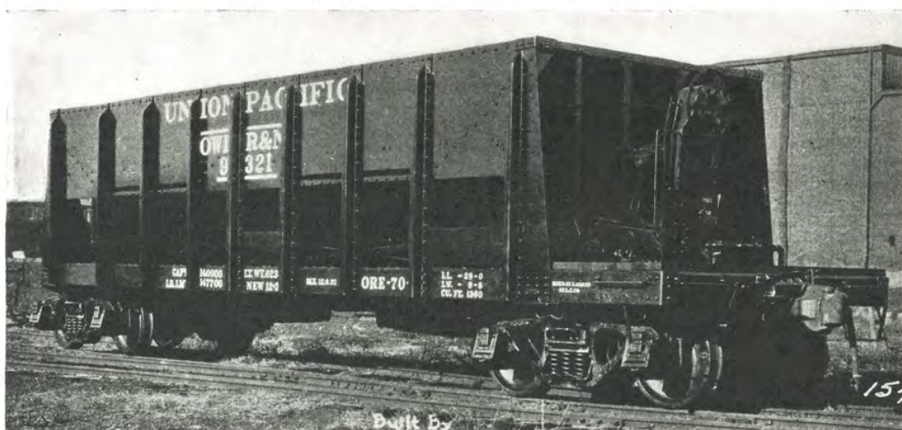
Fig. 2.672—Union Pacific (O-W. R. & N.) 70-ton ore car, AAR Class HMA. Builder, St. Louis Car Company.
