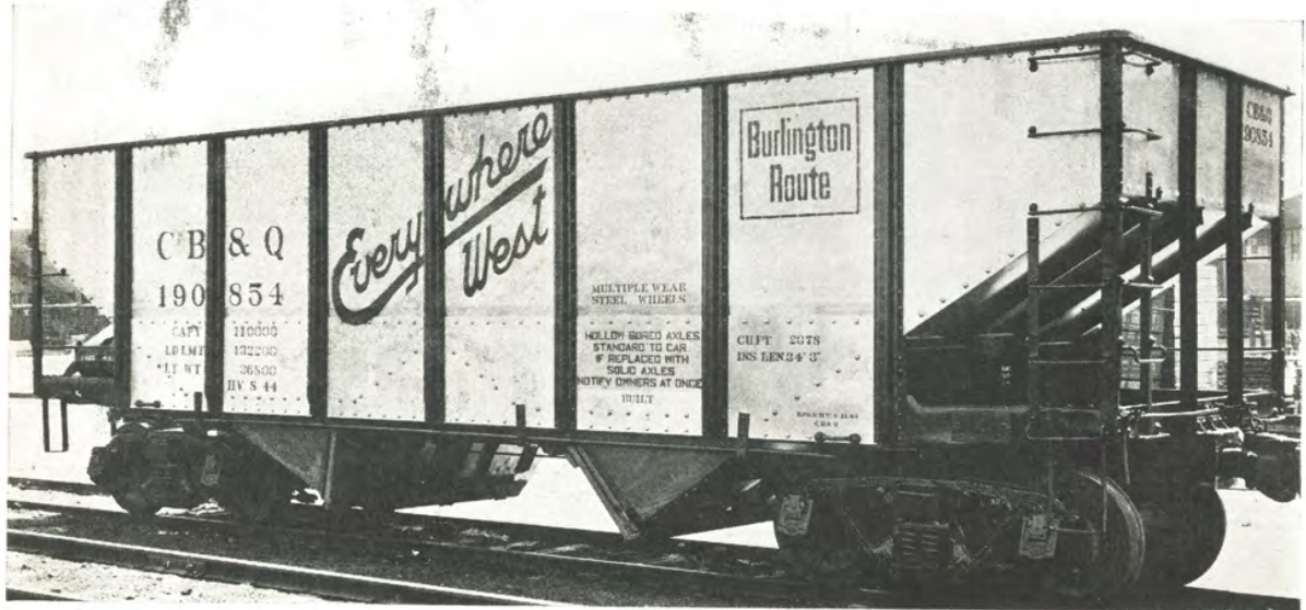
Fig. 2.615—C. B. & Q. 55-ton aluminum twin hopper coal car. Rebuilt on old steel frame. Built at Havelock shops. Light weight, 36,800 lb.; load limit, 132,200 lb.; capacity, 2,075 cu. ft.; inside, length 34 ft. 3 in.; width 9 ft. 6 in.; height of sides 10 ft. 9 in. Descriptions: Railway Mechanical Engineer, Sept. 1944; Railway Age, Sept. 9, 1944. (See also Page 267).
