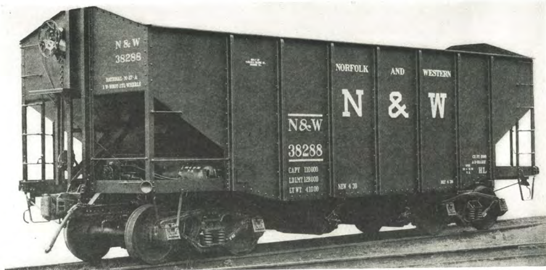
Fig. 2.605—Norfolk & Western 55-ton hopper car, Road Class HL, A. A. R. Class HM. Road Numbers 22,000-25,999; 38,000-39,999; 56,500-59,999; 67,000-69,999 (See also Figs. 2.604-2.607)
