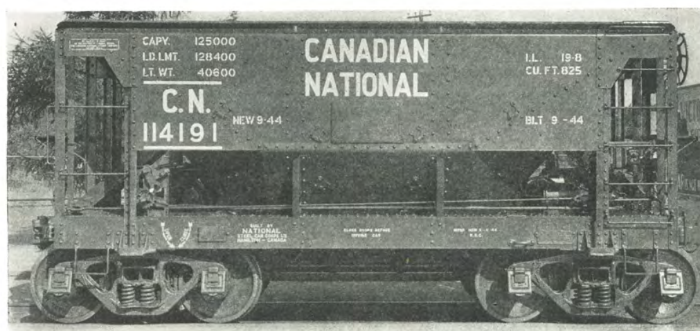
Fig. 2.673—Canadian National 50-ton center discharge ore car for use at Steep Rock mining operations. Built by National Steel Car Corporation, Ltd.
