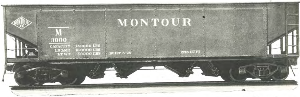
Fig. 2.611—Side view of 70-ton hopper car using Unitcast design cast steel body bolsters, crossbearers and hopper frames.
