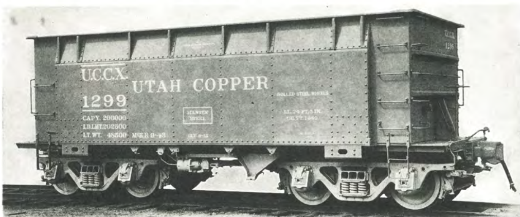
Fig. 2.671—Utah Copper Company 200,000-lb. capacity high-tensile steel, flat bottom, ore car. Unloaded by car dumper. Builder, Pressed Steel Car Company, Inc.
