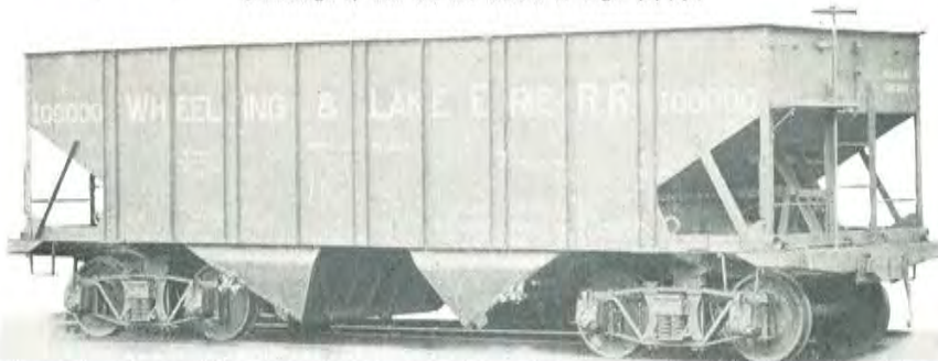
Fig. 51. Hopper Car, Structural Steel. Capacity, 100,000 lbs. Weight, 38,300 lbs. Standard Steel Car Co., Builders.
