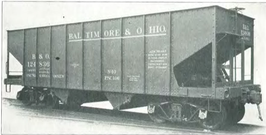
Fig. 50. Steel Hopper Car. Capacity, 100,000 lbs. Weight, 43,600 lbs. Pressed Steel Car Co., Builders. (Drawings of this car are shown in Figs. 424-429.)
