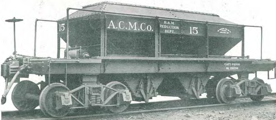
Fig. 2905—30-Ton Capacity Calcine Hopper Car. Builder, The Youngstown Steel Car Company.
