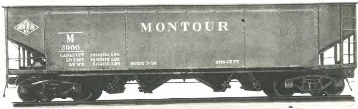
Fig. 2.611—Side view of 70-ton hopper car using Unitcast design cast steel body bolsters, crossbearers and hopper frames.
