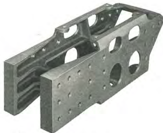
Combined Bolster Center Filler and Rear Draft Lugs A.A.R. Plate No. 534
