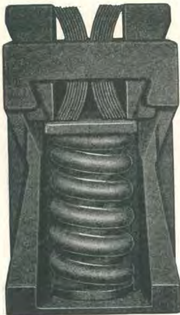
Cross-section of the 403 Gear showing spring arrangement
