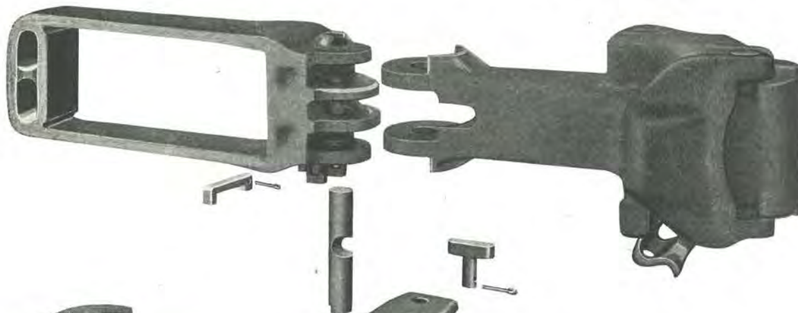
Fig. 10.100—Buckeye A.A.R. vertical-plane draft yoke of high-tensile steel.
