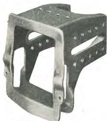
Fig. 10.102—Striker with Integral Front Lugs and Swing Coupler Carrier.
