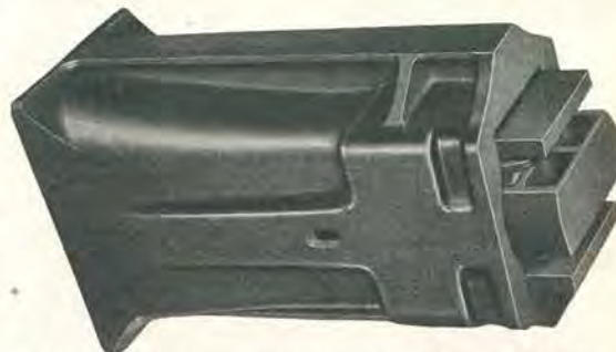
Westinghouse type NY-11-F draft gear, certified A.A.R.
