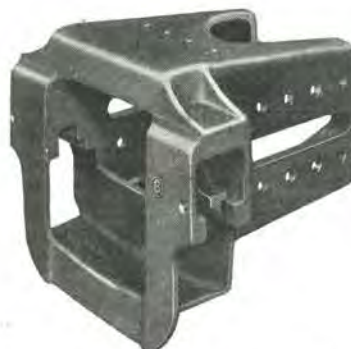
Fig. 10.103—Swing Motion Striker with Integral Front Lugs.
