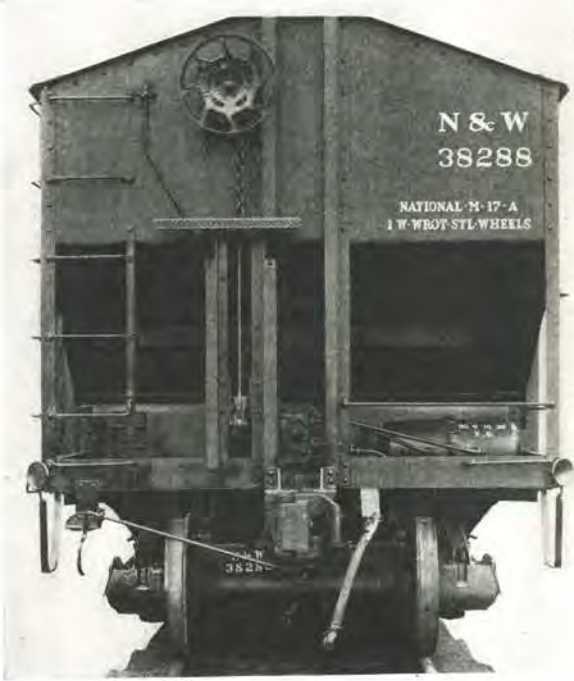
Fig. 2.607—Norfolk & Western 55-ton hopper car, Road Class HL.
