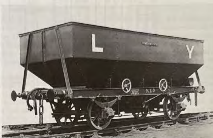
Left: Plate 209. Inside the unloading bay at Clifton in early 1915 with the far wagon showing the evidence of additional plating to raise the height of the side. Discharge was direct into the 50T capacity bunkers for each engine eliminating coal handling. Right: Plate 210. Ultimately all the Dia. 54 steel hopper wagons appeared like this. A May 1921 picture of revamped wagon No. 30785 with higher sides, vacuum standard turned down below the headstock, heavier duty buffers and flat-face axlebox covers. The loops attached to the solebar for rope/capstan haulage show up well.
