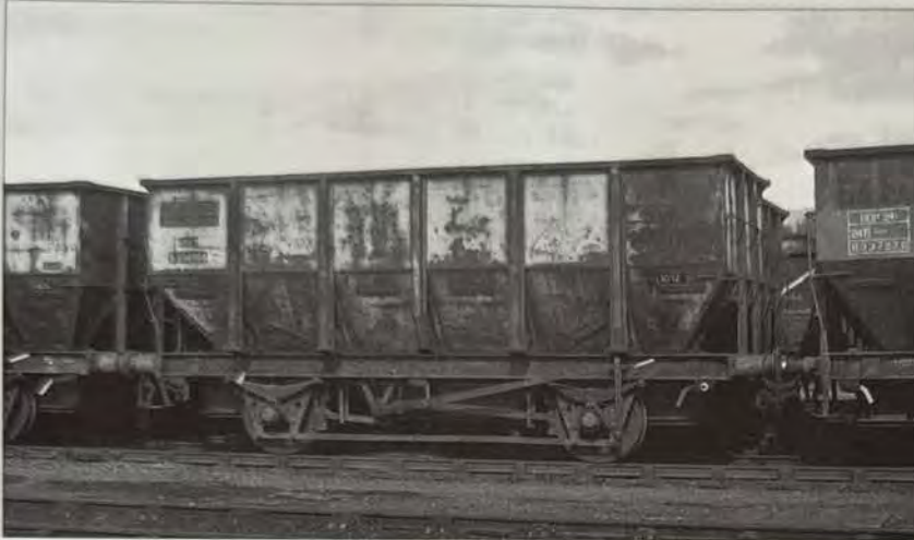
B336756N at Alloa, Scotland in November 1976. This lot 3426 wagon is in virtually original condition, albeit very weathered. It carries the original lettering panel for THORPE MARSH, and has received an "N" number suffix and the yellow triangle. Tare weight: 10ton 12cwt. (Author's Ref No W5997/DL)
