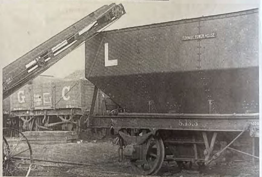
Plate 207. A posed shot at Clifton Junction Power Station in September 1919 with S35 Order wagon No. 30790 still lower height but redesigned for 'Clifton Power Station'. The wagon tared at only 7.19.1 and had a lovely repair on the nearest corner. Fully laden, its buffers seem dangerously lower than those of battery electric loco No. 2. NATIONAL RAILWAY MUSEUM
