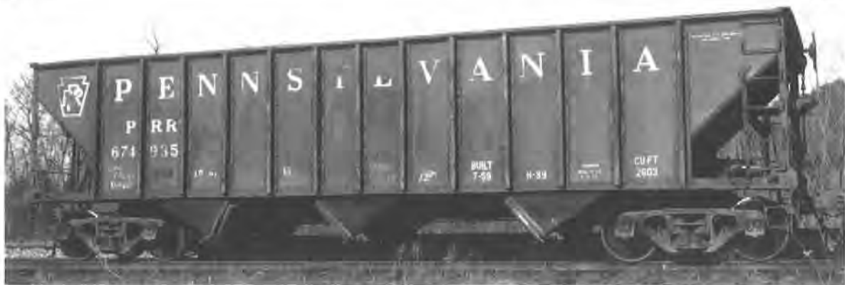
FIGURE 4.75 The H-39 class was the Pennsylvania Railroad's version of the "Committee Design" 70-ton hopper car, which was designed jointly by the Chesapeake & Ohio, Norfolk & Western, and Pennsylvania Railroads. The car had an internal capacity of 2,603 cubic feet. The Pennsy had over 16,000 hopper cars built in this series by a number of car builders. This car was built by American Car & Foundry in July 1959 and was seen here in Alexandria, Virginia, in December 1974. These cars can be identified by the thirteen riveted side posts. Note that the Pennsylvania design lacked the heap shields that are shown in the Norfolk & Western design in Figure 4.73. The Pennsy design employed Cor-Ten steel in all areas exposed to the lading in its cars of this series. [Courtesy: Bob's Photo]
