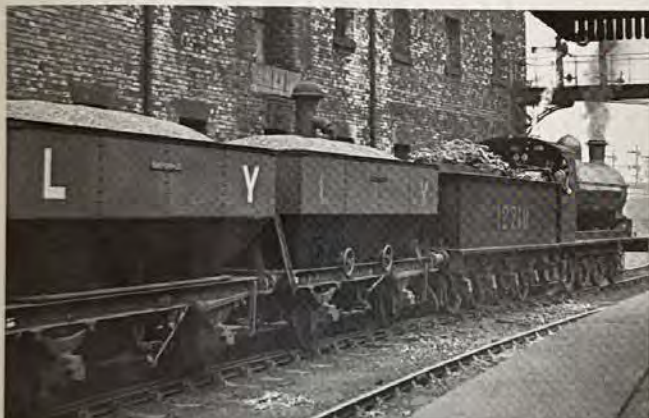
Left: Plate 209. Inside the unloading bay at Clifton in early 1915 with the far wagon showing the evidence of additional plating to raise the height of the side. Discharge was direct into the 50T capacity bunkers for each engine eliminating coal handling. Right: Plate 210. Ultimately all the Dia. 54 steel hopper wagons appeared like this. A May 1921 picture of revamped wagon No. 30785 with higher sides, vacuum standard turned down below the headstock, heavier duty buffers and flat-face axlebox covers. The loops attached to the solebar for rope/capstan haulage show up well.
