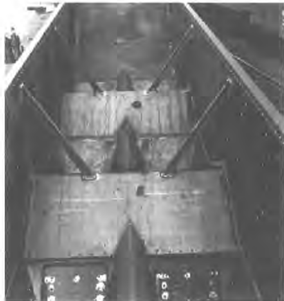
FIGURE 4.72 This is an interior view of a Norfolk & Western H-11-series hopper car, the railroad's 85-ton companion to the 70-ton "Committee Design" car. [Norfolk Southern Collection, Digital Library and Archives, University Libraries, Virginia Polytechnic Institute and State University; Courtesy: Norfolk Southern Corporation]
