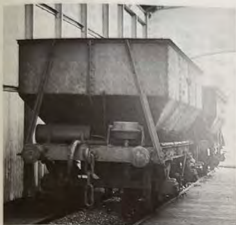
Left: Plate 209. Inside the unloading bay at Clifton in early 1915 with the far wagon showing the evidence of additional plating to raise the height of the side. Discharge was direct into the 50T capacity bunkers for each engine eliminating coal handling. Right: Plate 210. Ultimately all the Dia. 54 steel hopper wagons appeared like this. A May 1921 picture of revamped wagon No. 30785 with higher sides, vacuum standard turned down below the headstock, heavier duty buffers and flat-face axlebox covers. The loops attached to the solebar for rope/capstan haulage show up well.
