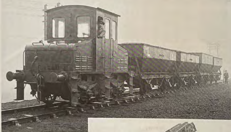
Plate 207. A posed shot at Clifton Junction Power Station in September 1919 with S35 Order wagon No. 30790 still lower height but redesigned for 'Clifton Power Station'. The wagon tared at only 7.19.1 and had a lovely repair on the nearest corner. Fully laden, its buffers seem dangerously lower than those of battery electric loco No. 2. NATIONAL RAILWAY MUSEUM
