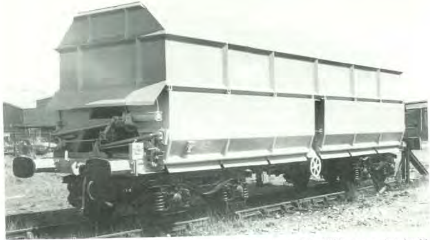
The first of the bogie gravel hoppers, FR 17001, was recorded at Fratton in May 1979 when newly painted in yellow ochre livery with white lettering and black running gear. The wagon was returning to Chichester after a visit to Eastleigh for tyre turning (R. Silsbury).
