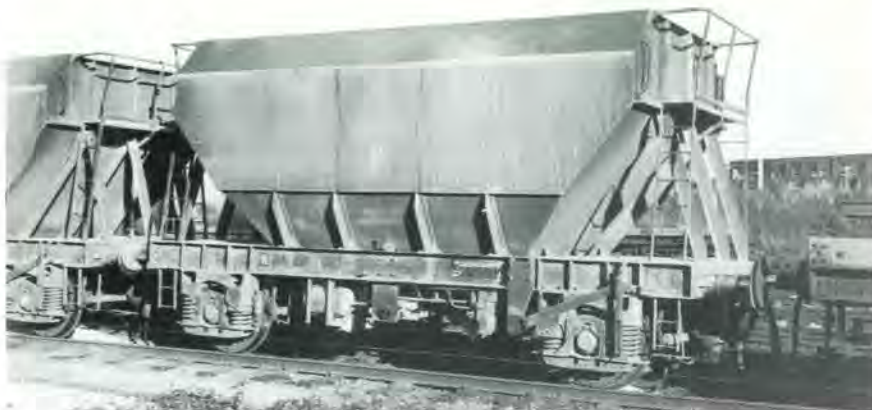
TAMC 14905 is another 51 t aggregate hopper built by Standard Wagon, but in this case owned and operated by Tarmac Roadstone. These vehicles, which have a more 'chunky' appearance than earlier hoppers, normally run in block-train formations, although this example was recorded at Warrington in August 1987 when en route to works for routine maintenance.
