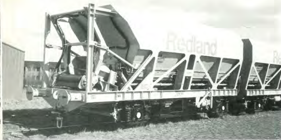
REDA 16200, a 'Self-Discharge Hopper Train' 'outer' wagon. Note the conveyor belt which is extended beyond the headstock when unloading. This train is particularly suitable for short-term traffic flows as it can be unloaded without the need for any on-site facilities other than a rail siding. Body and solebars are pale green; the 'Redland' name is red, while other lettering and suspension units are black. Heywood, April 1988.
