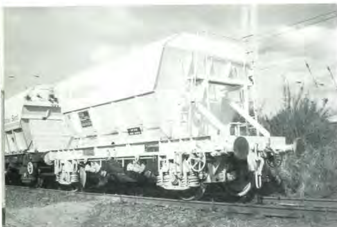
As detailed in the text, a number of the British Steel Teesside hoppers have been rebuilt for general aggregate traffic. One such vehicle, SRW 18509, was recorded at Warrington in September 1987 sparkling in its new overall white livery with 'Railease' in blue and other lettering in white on black patches.
