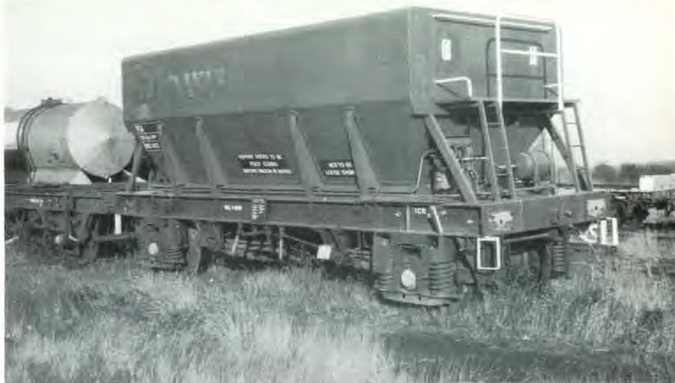
The unique 51 t aggregate hopper built by W.H. Davis, DAVS 14433, photographed when stored out of use at Shirebrook in November 1985. By this date it was painted red with black 'Davis' symbol and underframe.
