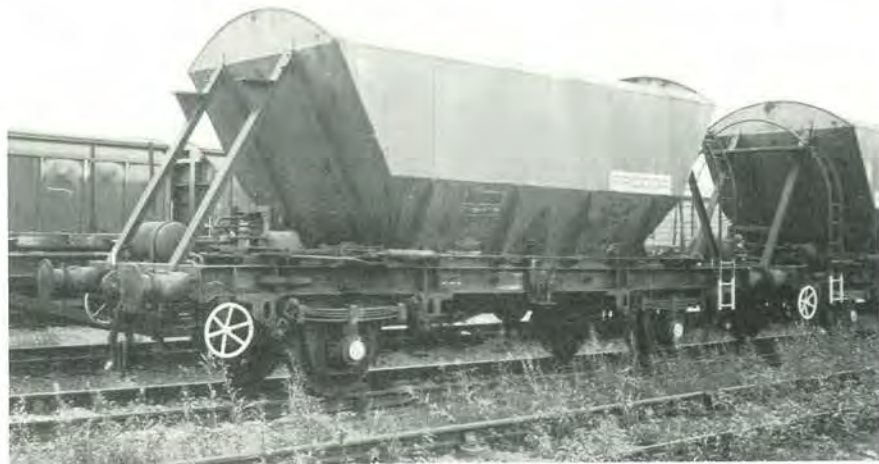
Above This re-sprung salt hopper PR 8230 was recorded at Tees Yard in September 1987. Livery is rusty yellow with the 'Procor' symbol in blue and white, white lettering on black patches and black underframe.
