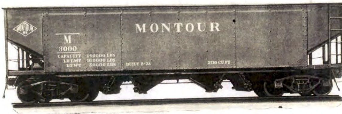
Fig. 2.611—Side view of 70-ton hopper car using Unitcast design cast steel body bolsters, crossbearers and hopper frames.
