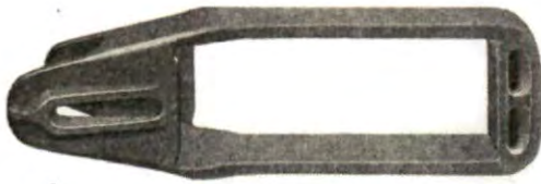
Fig. 10.99—Buckeye A.A.R. vertical-plane draft yoke for 24 \frac{5}{8} in. friction gears.
