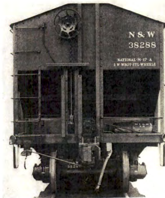
Fig. 2.607—Norfolk & Western 55-ton hopper car, Road Class HL.
