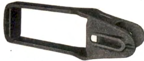
Fig. 10.100—Buckeye A.A.R. vertical-plane draft yoke of high-tensile steel.
