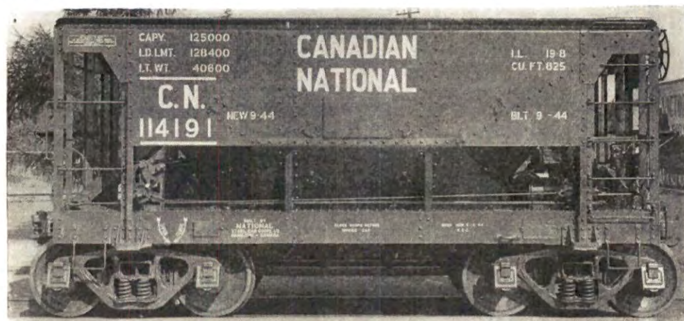
Fig. 2.673—Canadian National 50-ton center discharge ore car for use at Steep Rock mining operations. Built by National Steel Car Corporation, Ltd. Light weight, 40,600 lb.; load limit, 128,400 lb.; capacity, 825 cu. ft.; length inside, 19 ft. 8 in. * (See also page 294)
