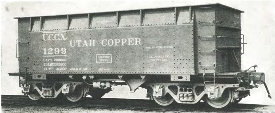
Fig. 2.671—Utah Copper Company 200,000-lb. capacity high-tensile steel, flat bottom, ore car. Unloaded by car dumper. Builder, Pressed Steel Car Company, Inc. Light weight, 48,500 lb.; load limit, 202,500 lb.; capacity, 1,640 cu. ft.; inside, length 24 ft. 5 in.; width 10 ft. 6 in.; height 6 ft. 6½ in. Description of earlier lot: Railway Age, October 30, 1937
