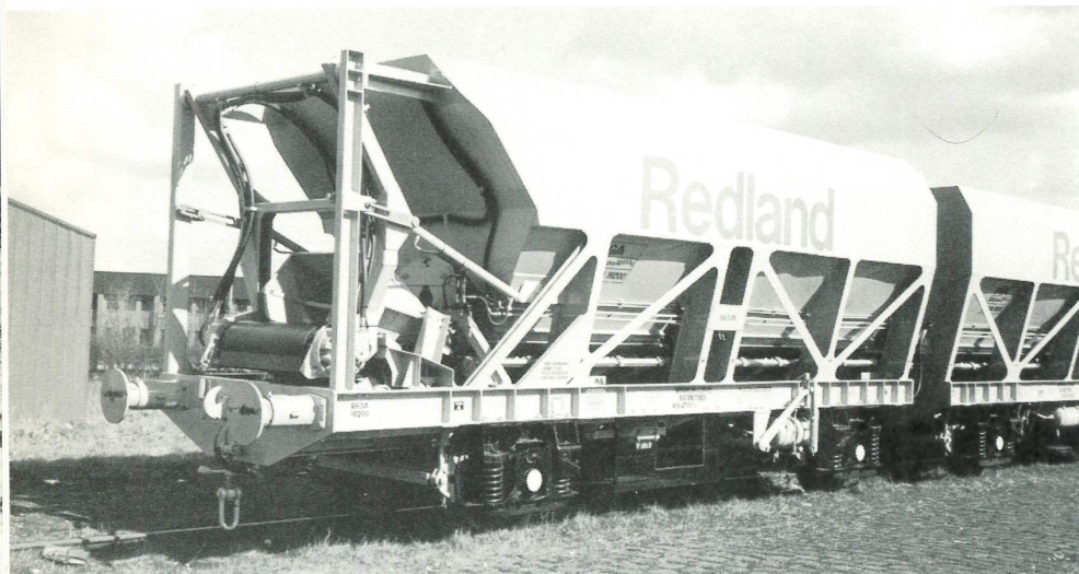
REDA 16200, a 'Self-Discharge Hopper Train' 'outer' wagon. Note the conveyor belt which is extended beyond the headstock when unloading. This train is particularly suitable for short-term traffic flows as it can be unloaded without the need for any on-site facilities other than a rail siding. Body and solebars are pale green; the 'Redland' name is red, while other lettering and suspension units are black. Heywood, April 1988.
