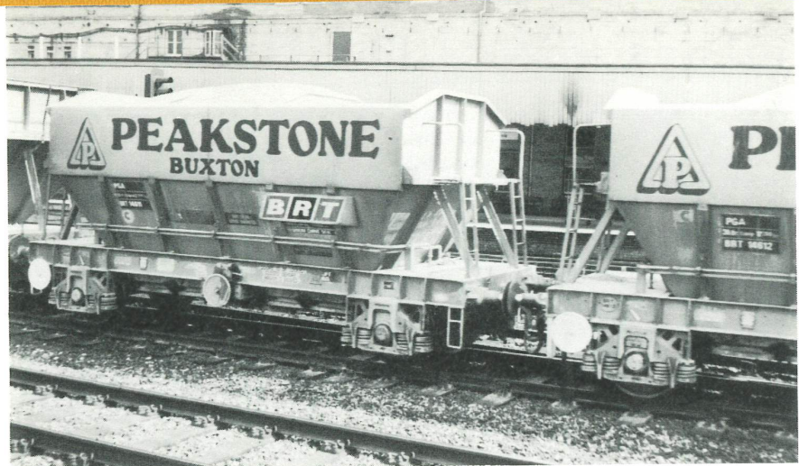
BRT 14611 is one of the 51 t aggregate hoppers leased to Peakstone of Buxton. Note the straight-channel solebar, preferred by the builders Standard Wagon, and the attractive livery which comprises mustard body and underframe, with black 'Peakstone' lettering and symbol, 'BRT' symbol in red, black and white, and other lettering white, some on black patches.
