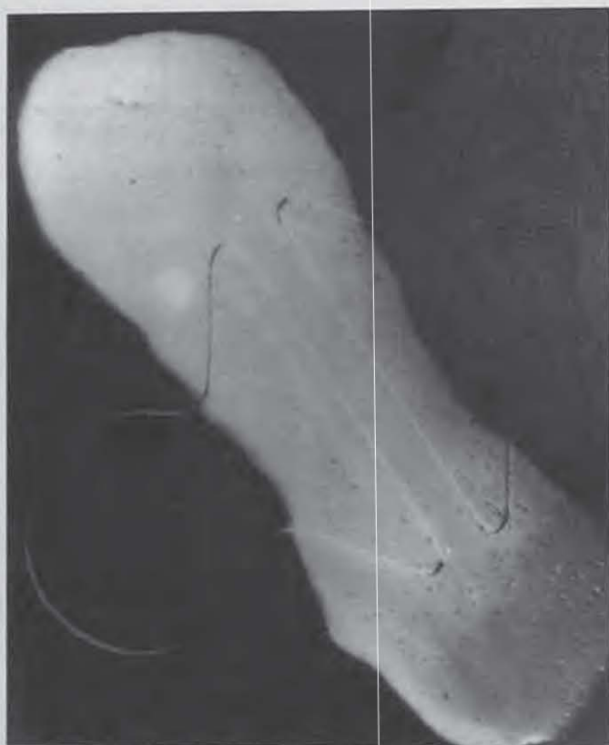
Figure 1.3 The first metal-oxide-semiconductor field-effect transistor. 13 (Photograph courtesy of Bell Laboratories.)
