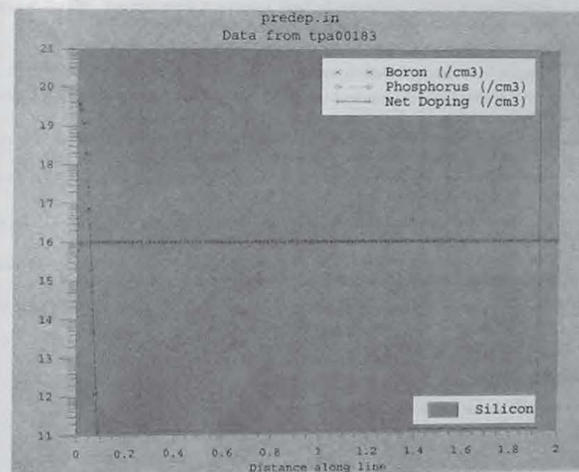
Figure 6.13 Plot of boron concentration as a function of depth into the silicon substrate, using SUPREM.
