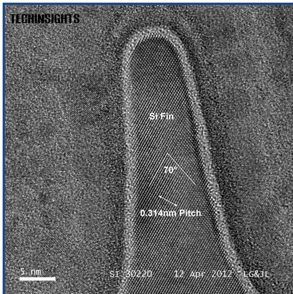
Figure 2.1.6: Silicon fin of a PMOS transistor, HRTEM lattice-fringe image.
