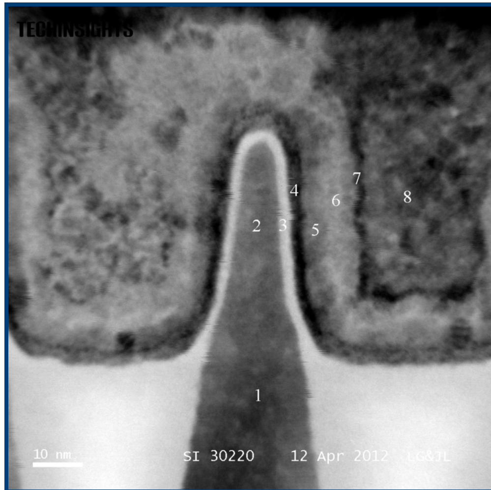
Figure 2.3.2.8: PMOS transistor, TEM cross-section along metal gate with EDS sites annotated.
