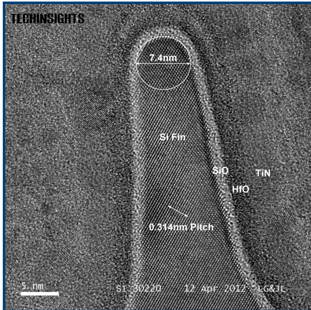
Figure 2.3.2.4: Middle part of the PMOS transistor fin with gate dielectric and metal gate layers, HRTEM image.
