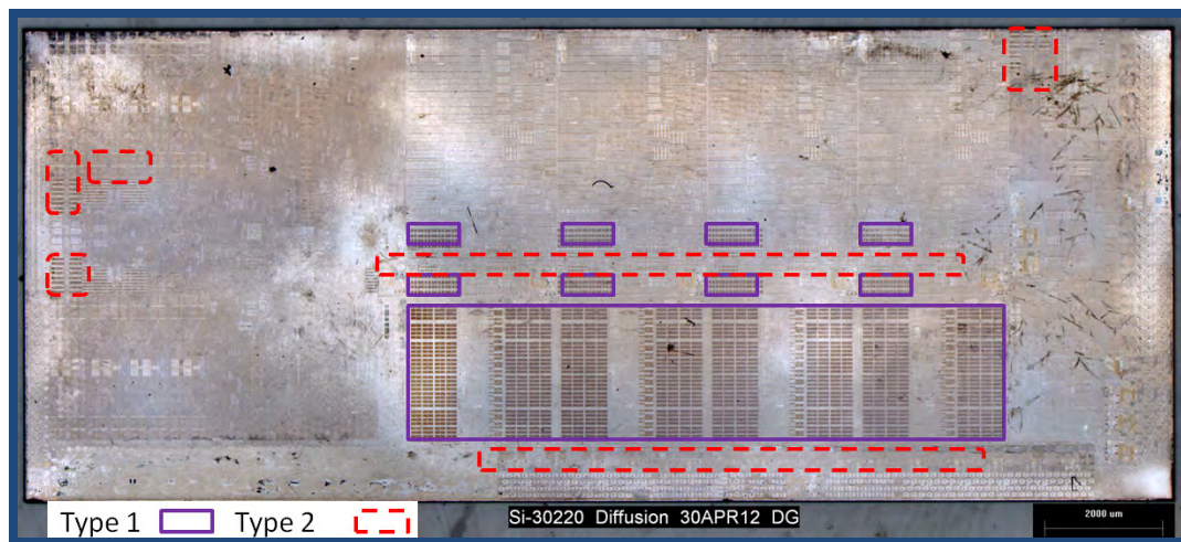
Figure 3.1.3: Die de-layered to diffusion. The approximate location of SRAMs is marked.
