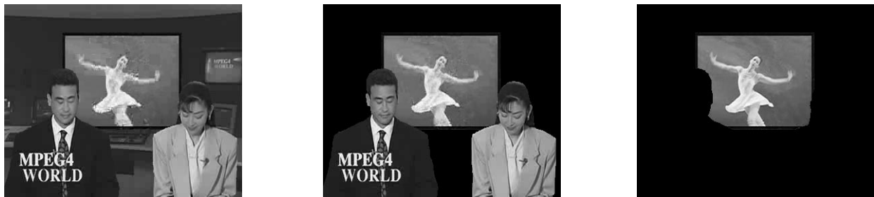
Fig. 13: Illustration of adaptable transcoding of News sequence with key object identification, 384 -> 128kbps. The motion intensity and difficulty hints are used to order the importance of each object and the difficulty hint alone is used for bit allocation. Fewer objects can be delivered with noticeable higher quality.
