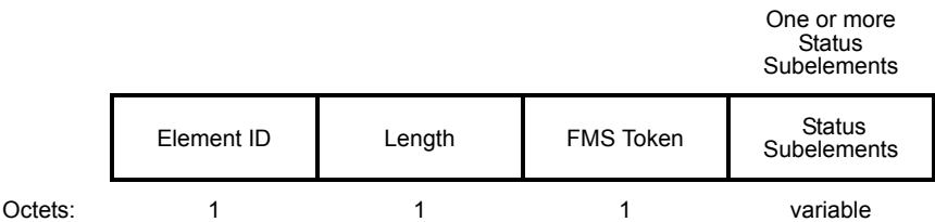
Figure 8-328—FMS Response element format
