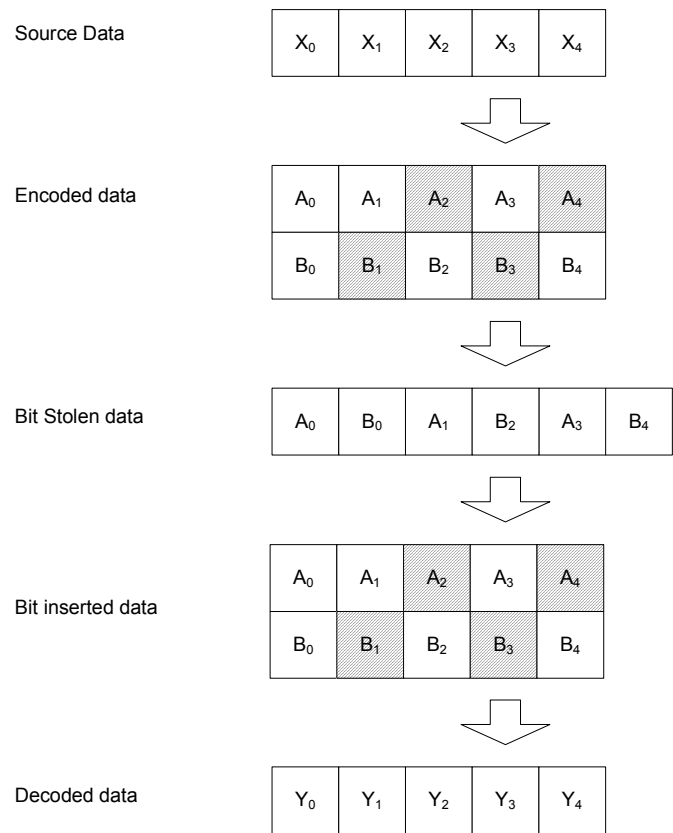
Figure 20-11—Puncturing at rate 5/6
