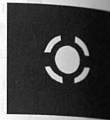
Fig. 12.16 Solder relief area around pads
