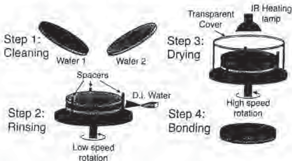
Fig. 11-22 Schematic of the microcleanroom setup and procedure.
