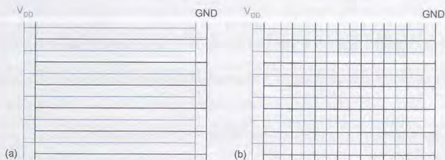
FIG 9.47 Power supply network
