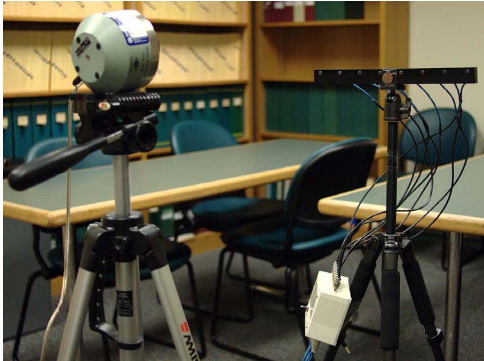
Figure 2.2: Impulse response measurement setup: mouth simulator (B&K Type 4227), a linear microphone array with a penny in the center, and eight channel self-made pre-amplifier (circuit diagram and interior are shown in Appendix D.)
