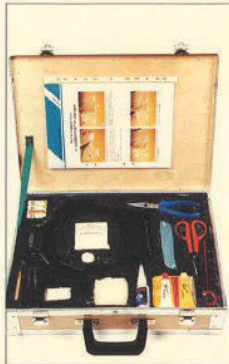
The simple box that helps the operator connect a felt with a seam.
