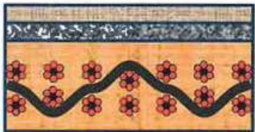
Extra fine cap over medium denier intermediate layer with coarse fibers surrounding base fabric
