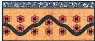
Fine denier cap over coarse fibers
