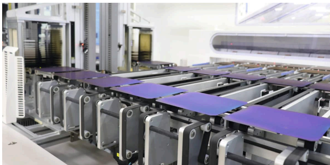
Jolywood solar cell production line
