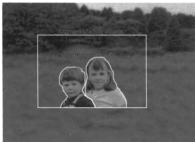
Figure 4.19 Example of background sprite and foreground VOPs
