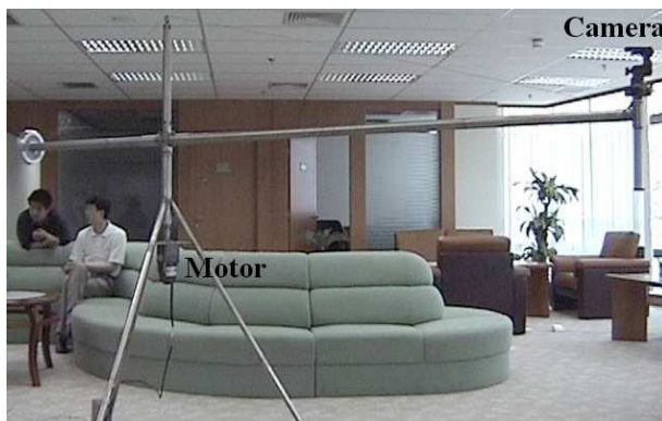
Fig. 4.9 Camera setup for acquiring Concentric Mosaics (CMs). The camera is counterbalanced by a weight; during image acquisition, it is rotated by a motor at a constant rotational speed.
