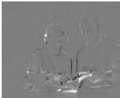
Figure 3.13 Residual : 16 \times 16 block size
