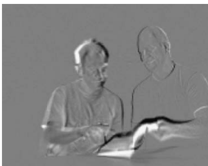
Figure 3.12 Residual : no motion compensation
