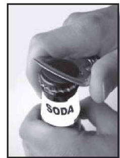
A Bottle Opener is a Second-Class Lever
