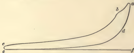
FIG. 1-34. — Diesel Engine Diagram.
