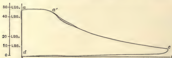
FIG. 1-32. — Diagram from Brayton Working Cylinder.
