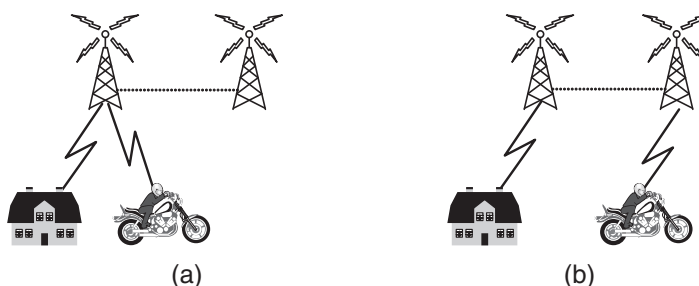
Figure 1-32. Mobile phone handover (a) before, (b) after.
