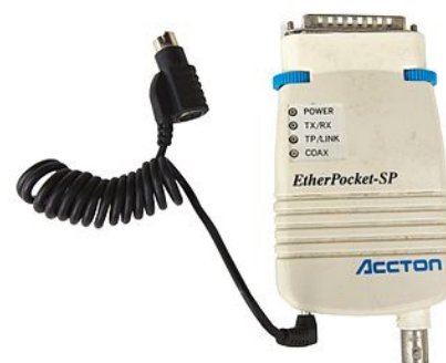
Accton Etherpocket-SP parallel port Ethernet adapter (circa 1990). Supports both coaxial (10BASE2) and twisted pair (10BASE-T) cables. Power is drawn from a PS/2 port passthrough cable.
