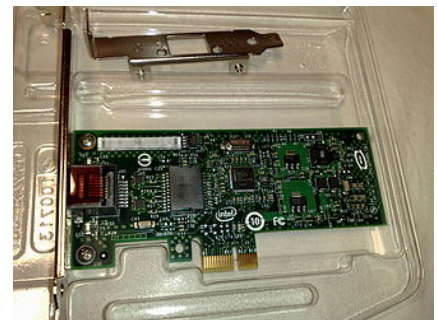
An Intel 82574L Gigabit Ethernet NIC, PCI Express ×1 card
