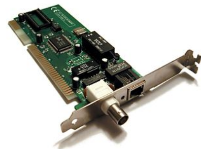
A 1990s ISA network interface card supporting both coaxial-cable-based 10BASE2 (BNC connector, left) and twisted pair-based 10BASE-T (8P8C connector, right)
