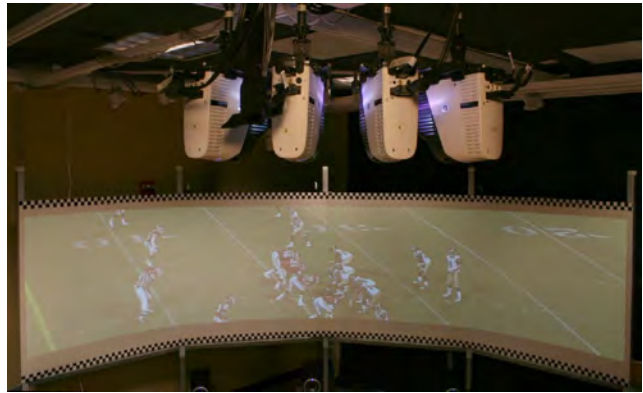
Figure 1. Projector array, curved screen, and example imagery, with lights on. A vertical physical seam exists at center of screen.
