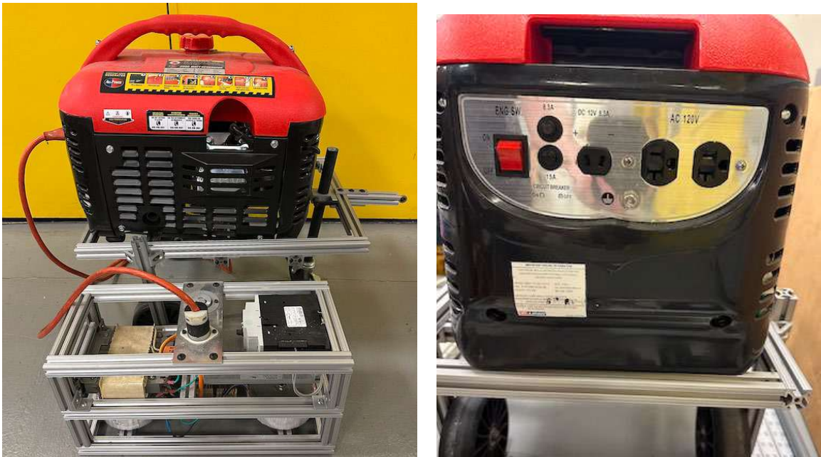
Portable Generator for Robotic Mobile Boom Crane.
