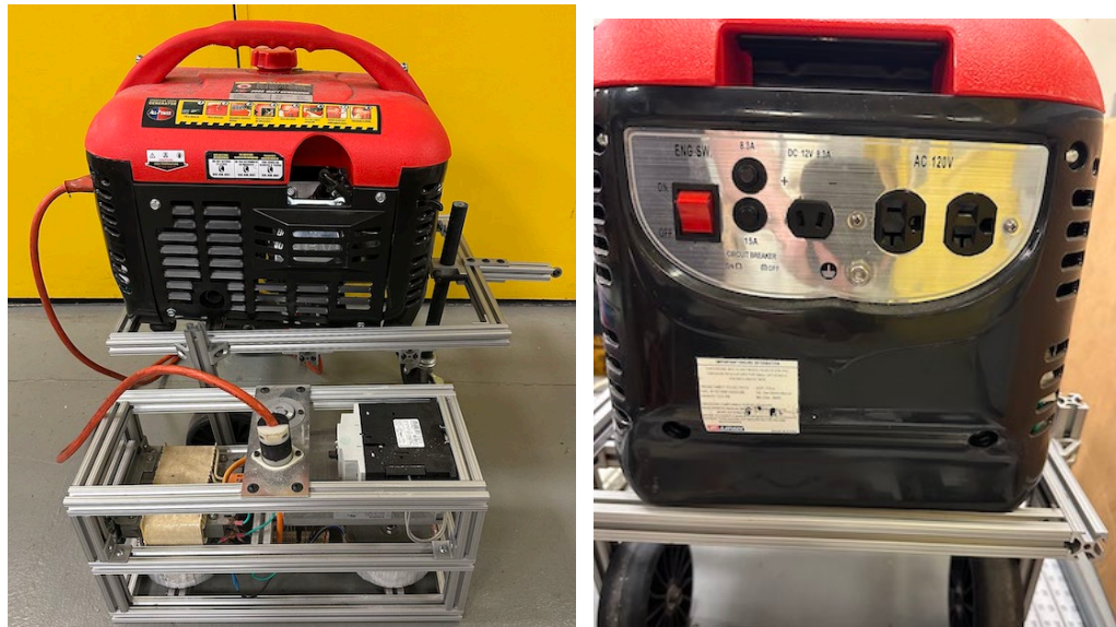
5 6 7 8 9 10 11 12 13 14 15 Generator for Robotic Mobile Boom Crane.
