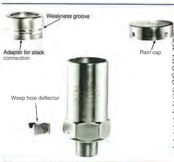
EXHIBIT 5.22 External-Type Pressure Relief Valve for Older, Small ASME Container. (Courtesy of Engineered Controls International, Inc.)
