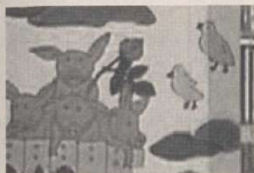
Fig. 12. Enhanced to progressive SDTV, Mobcal at 5 Mbs/s. Part of the I-picture (frame 24, top field). PSNR = 30.1 dB.
