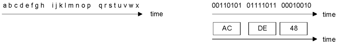
Figure 11—IEEE 802.3, etc., frame: Order of bit and octet transmission for an OUI
