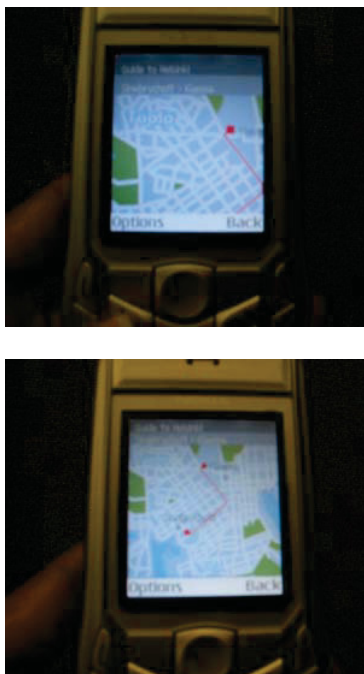
Figure 7: Camera-based interaction in a map viewing application. The map is rendered using vector graphics, so it can be scaled with no loss in quality. Physically-based scrolling and zooming coupled with vector graphics creates a better navigation experience for users.
