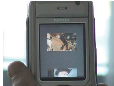
Figure 6: Picture browser application. In this prototype, a large collection of photographs is presented. The user can move their phone to scroll through the collection. If they slow down their movement, the application automatically adjusts the zoom level to help the user browse.
