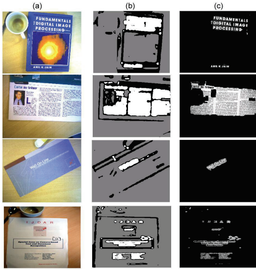
Figure 3. (a) Original images (b) Three-classes clustering (c) Text region
